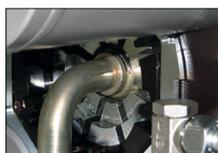
The SC 12 series can be used to crimp short 90° elbow fittings with a long drop. This is impossible for other conventional machines.
