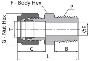
The E dimension refers to the smallest nominal orifice. It might be larger at tapered thread end, straight thread end.
