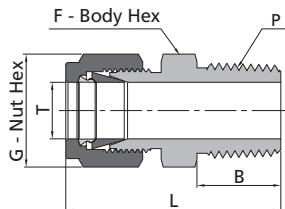
1. The T dimension refers to the smallest nominal orifice. It might be larger at tapered thread end, straight thread end.
